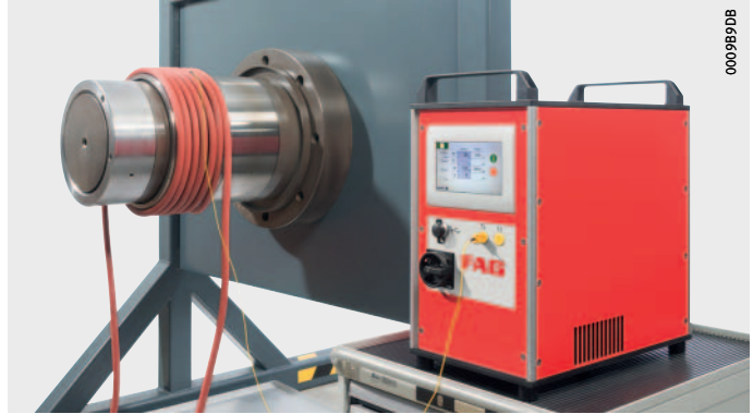
Figure 2 Induction heating of inner ring
